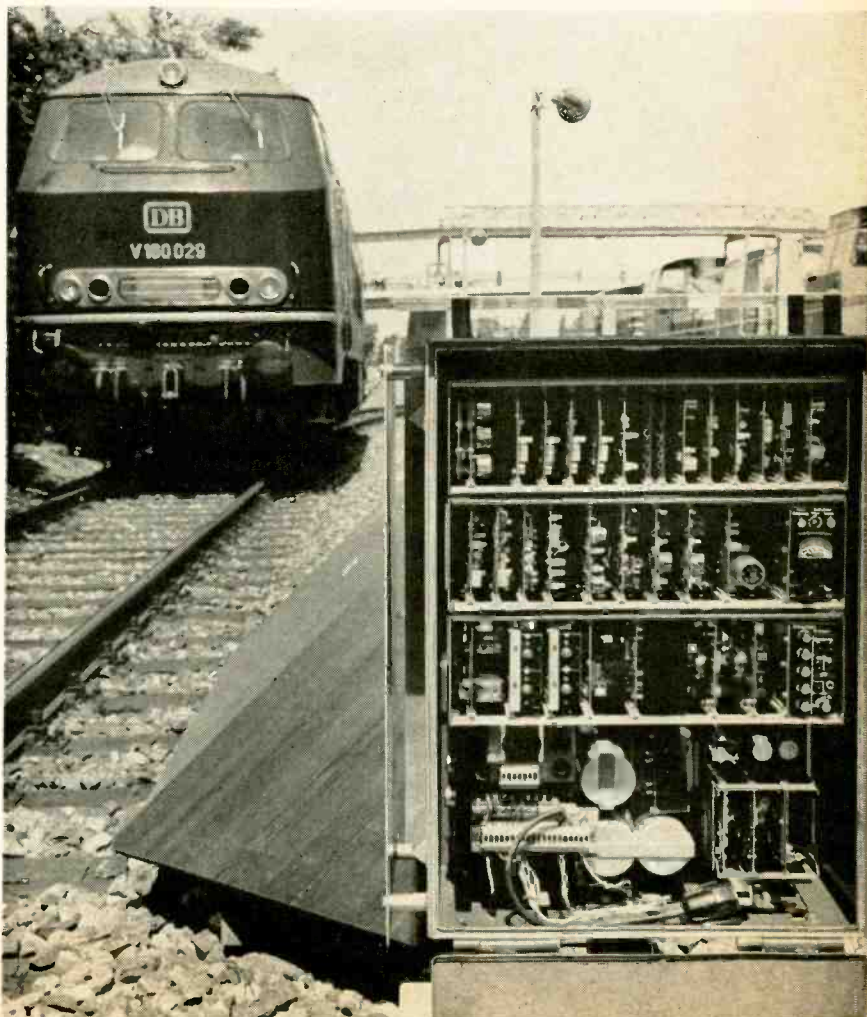
Railroad reader. When car passes automatic reader at right, numbers stored in transponder on car are inductively coupled to reader. Car numbers can be punched onto tape or written out on a typewriter at monitoring station.
