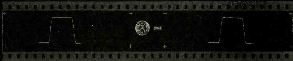
Typical single-shot photo of fast risetime pulses recorded on 977 Fiber Optic Oscilloscope using Type 2475 film.
