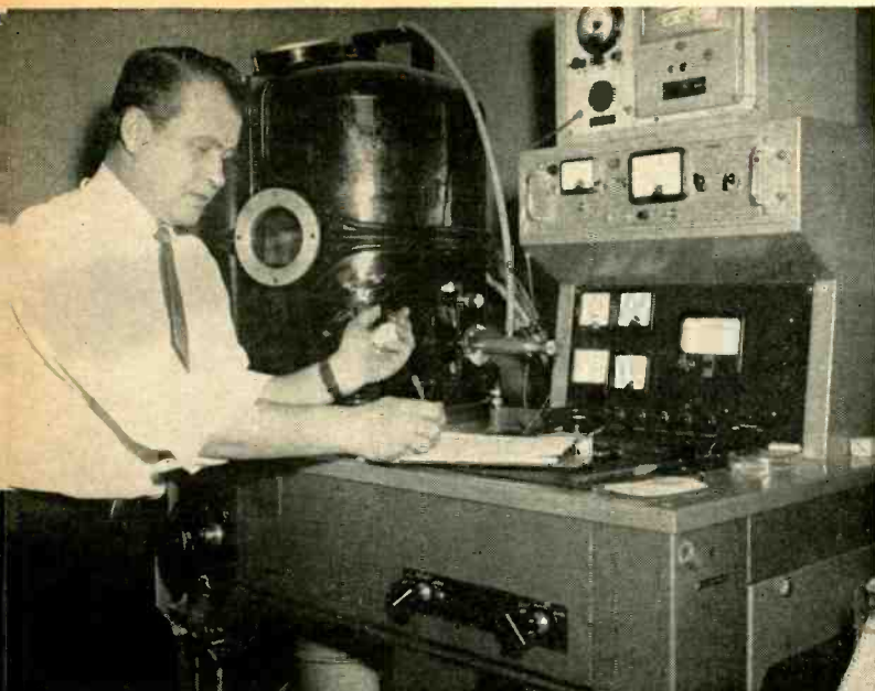
Research engineer Harry Bajars times the wafer metal bonding-layer deposition, accomplished by sputtering from a sheet cathode in a chamber containing argon.
